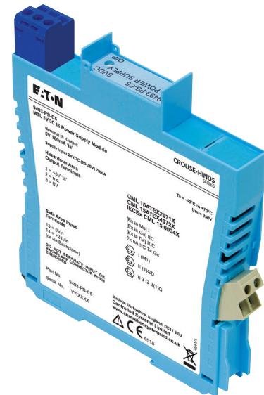
**The 9493-PS-XXX Power Supply is a general purpose Intrinsically Safe power supply unit.** It takes a 24V DC safe area or Zone 2 supply and produces an Intrinsically Safe output available in a range of different DC voltages. The 9493-PS-XXX may be mounted in a safe area or Zone 2 hazardous area.
